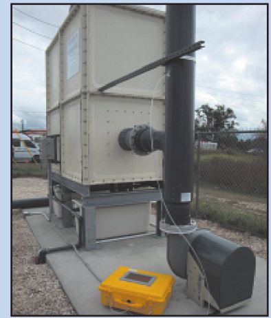
Bag sample collection at outlet stack
